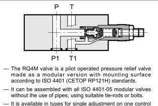
It is available in types for single adjustment on one control line or dual on two control lines and with four different pressure adjustment ranges.
